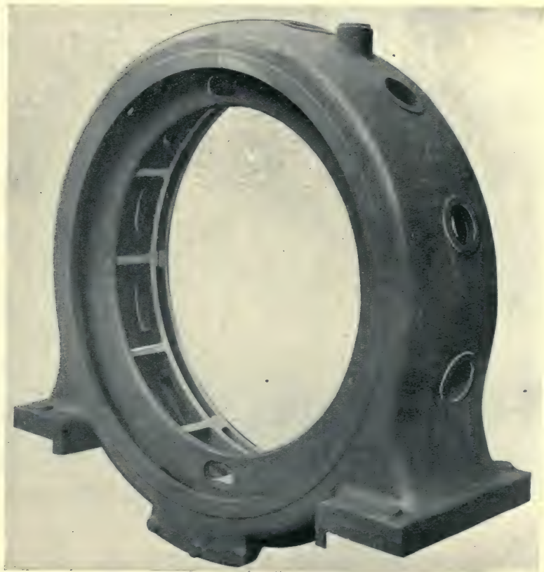
FIG. 65.—Casting for Frame of Stationary Armature. Scott & Mountain.
